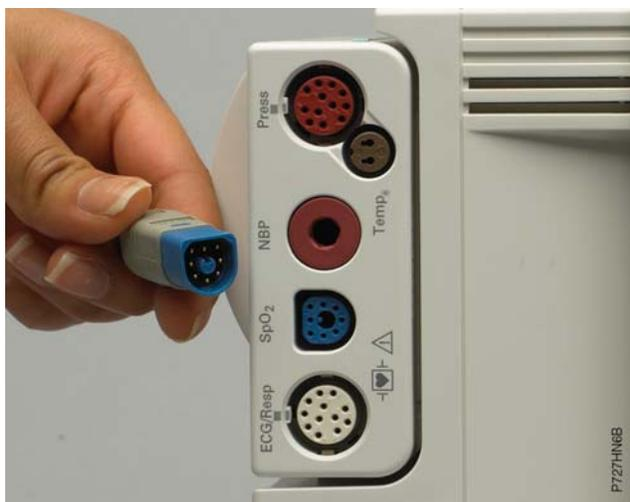
**An additional level of protection.** Not only is the plug physically compatible with just one of the jacks, but it is also color coded to further prompt users to make the correct connection. This is a good example of using multiple levels of equipment design solutions.
