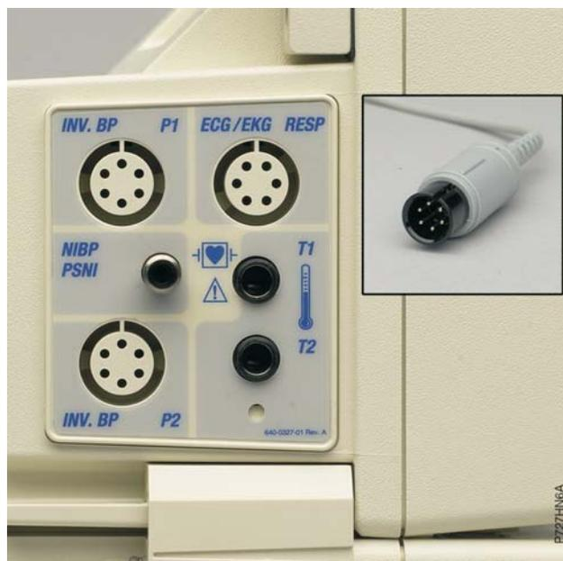
**The value of keyed connectors.** Although the three jacks look almost identical, the plug shown in the inset can only attach to the top right-hand jack because of the position of the pins and the slot in the plug. Thus, even if a clinician tries to insert the plug into the wrong jack, the connection won’t be possible.
